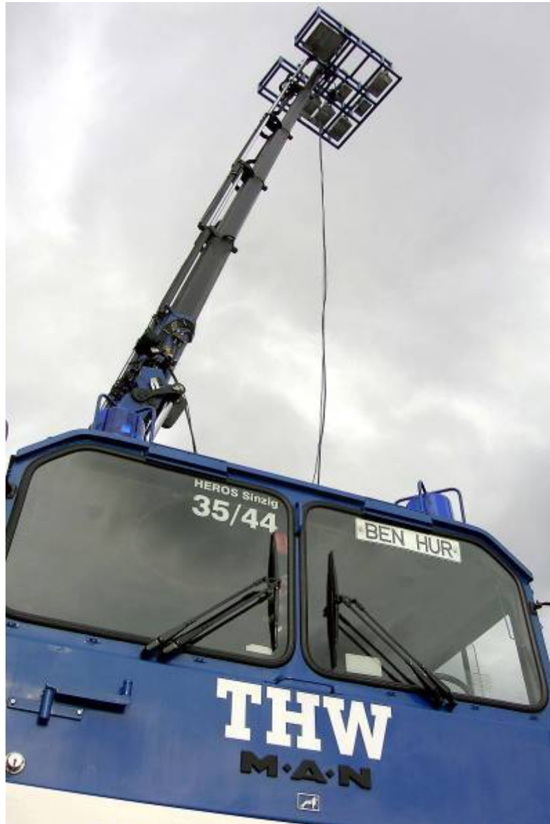
Selfmade lighting cross-beam for a MAN crane
