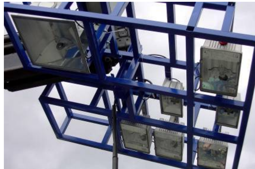
Selfmade lighting cross-beam for a MAN crane
