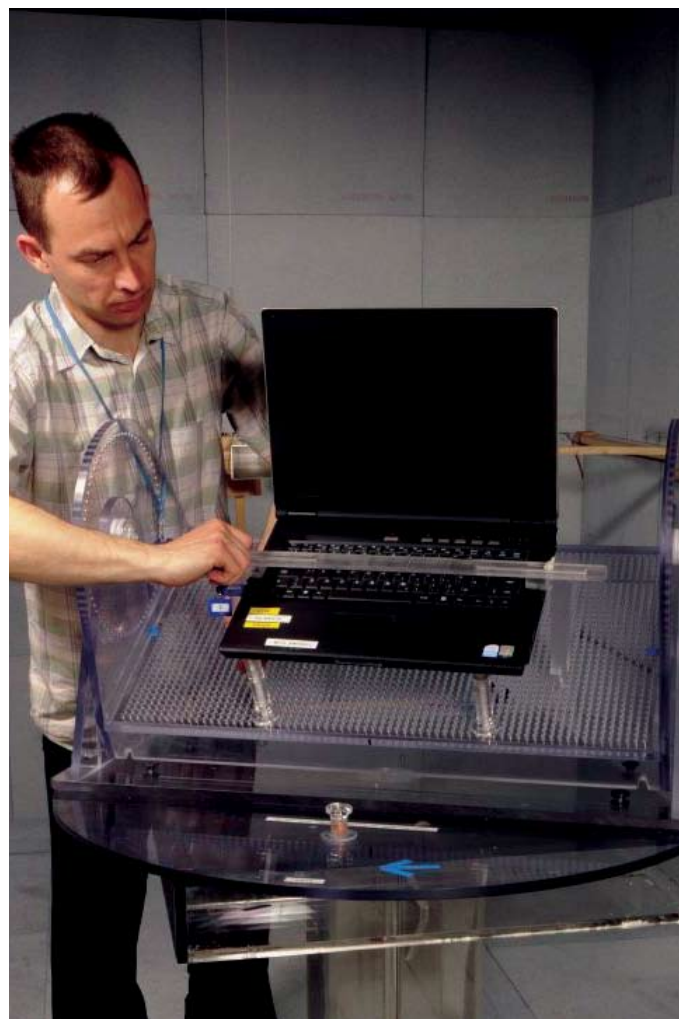
The manual positioning system rotates in azimuth and elevation directions in 30° steps Photo: HPA
