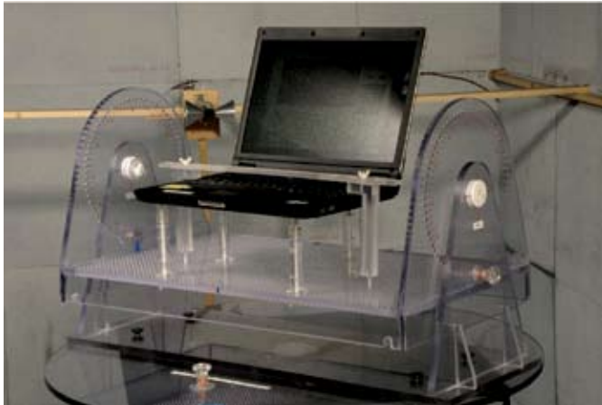
Setup for assessing the electric field distribution around a laptop, EMF laboratory, HPA Chilton site Photo: HPA
