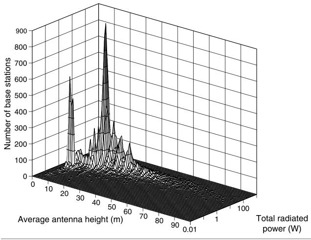
Fig. 1.10 Distribution of 32 837 base stations in the United Kingdom according to average antenna height and total radiated power
