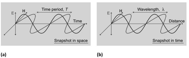
E, electric field; H, magnetic field. Prepared by the Working Group
