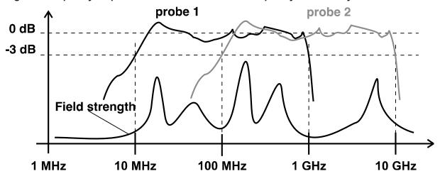
Fig. 1.16 Frequency response of two broadband radiofrequency field-survey meters
