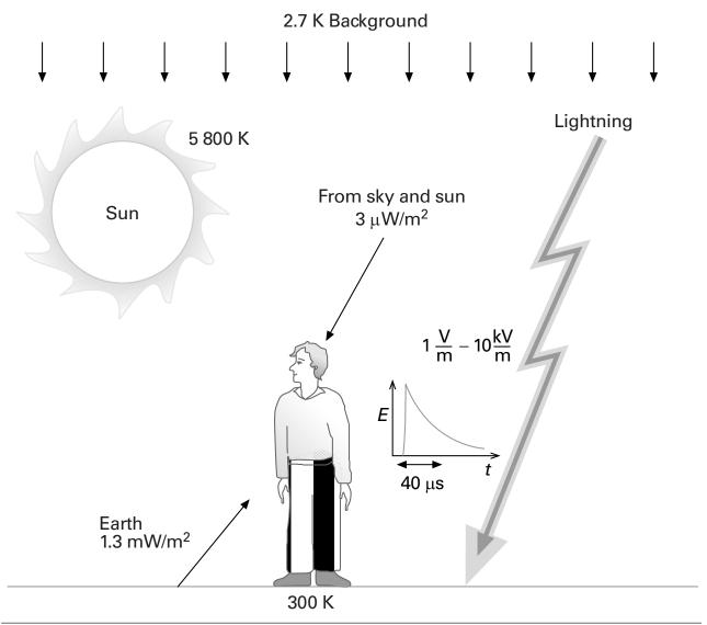
Fig. 1.3 Terrestrial and extraterrestrial sources of radiofrequency radiation
