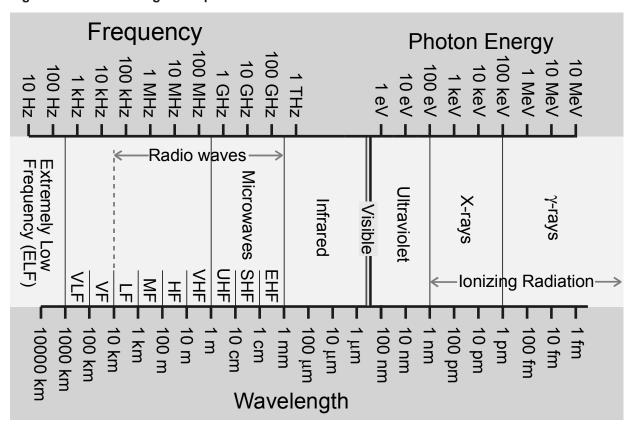
Fig. 1.2 The electromagnetic spectrum
