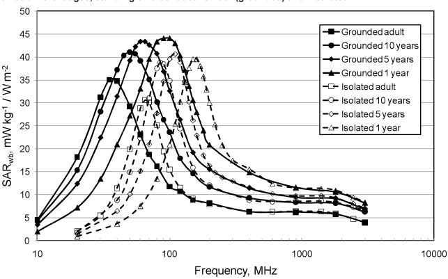
Fig. 1.12 Variation in the whole-body specific absorption rate (SAR) produced per unit power density as a function of frequency in the adult male phantom NORMAN, and child phantoms of three different ages, standing on a conductive floor (grounded) and insulated
