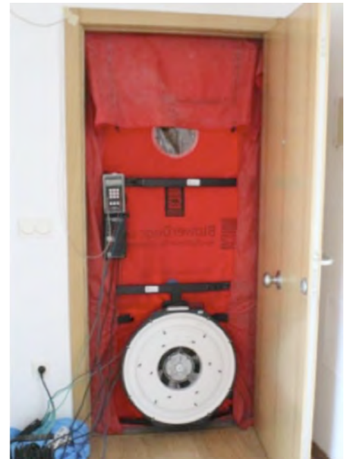
Assembly of the blower door
