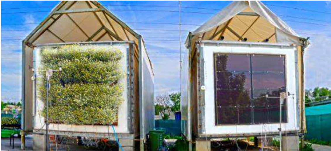
Fig. 3 PASLINK test site in the LCCE. From left to right: ILARGI cell with a vegetable facade sample, EGUZKI cell with a ventilated photovoltaic sample.
