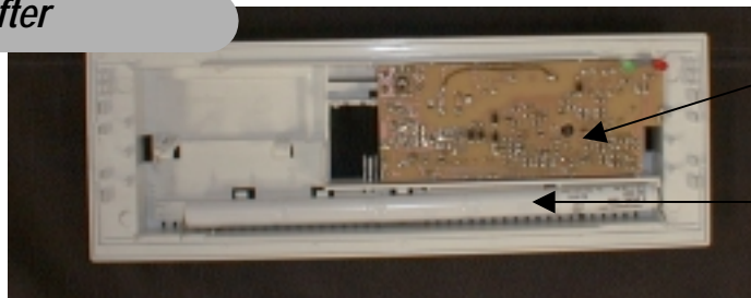
Figure 7.- Comparison of the HYDRA product before and after the Ecodesign project. As may be seen, the printed circuit is smaller and does not contain halogenides and the battery has been replaced by a better one from the environmental point of view.
