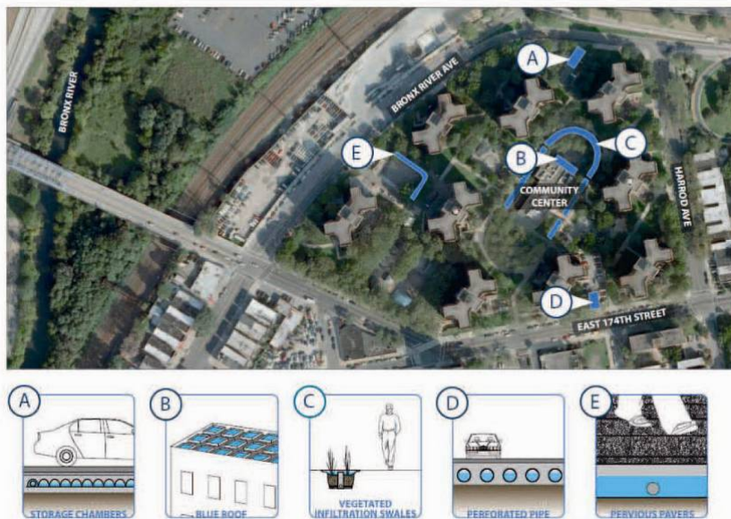
Figure 20: Pilot - Model High Density Housing Retrofit
